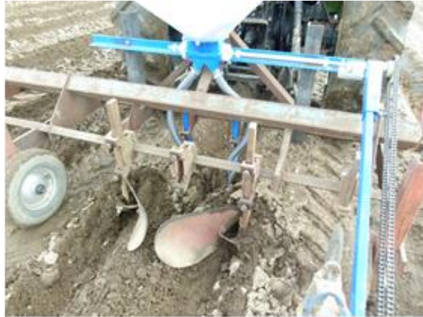
Figure 2. Horstine applicator, modified to place fertilizer in the furrow with the asparagus crowns.
